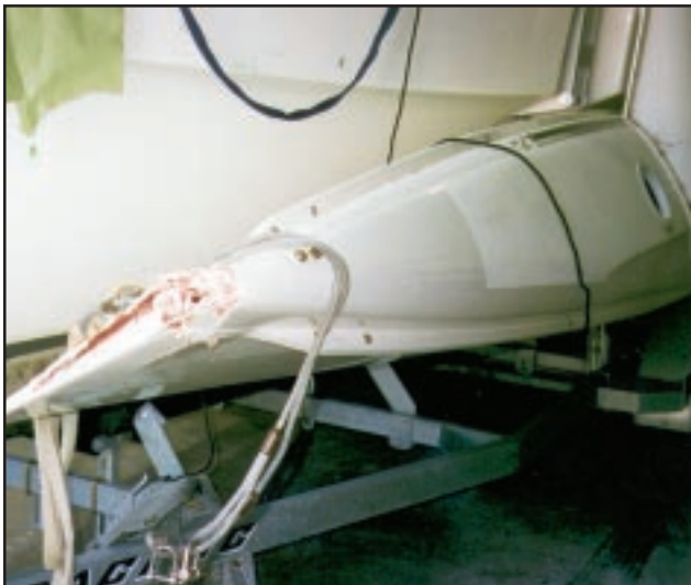
Extensive damage to bow can be seen, plus cracks in fwd. beam
